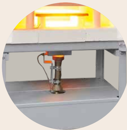
15 kW propane gas mounted under the kiln
