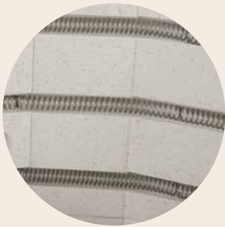
All-round heating elements, protected in grooves
