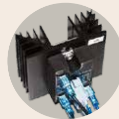
Solid state relays ensure low-noise heater operation
