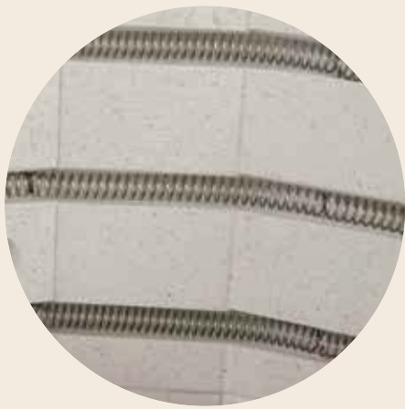
All-round heating elements, protected in grooves
