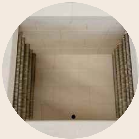
Heating elements on support tubes on both sides ensure uninterrupted heat radiation
