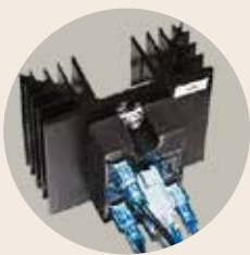
Solid state relays ensure low noise heater operation
