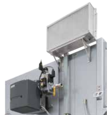
Direct gas-firing at a chamber dryer
