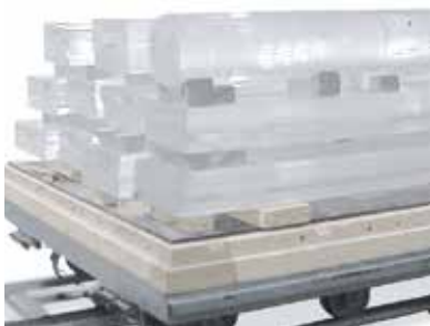
Bogie hearth furnace for tempering quartz rods
