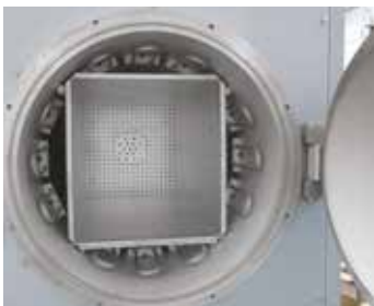
Inside heating in retort furnaces NRA ../06
