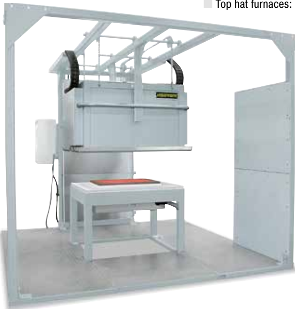
Top hat furnace H 240/S. Table accessible from four sides for welding quartz glass constructions by vertical and horizontal moveable top hat
