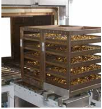
Continuous furnace for bulk materials in baskets
