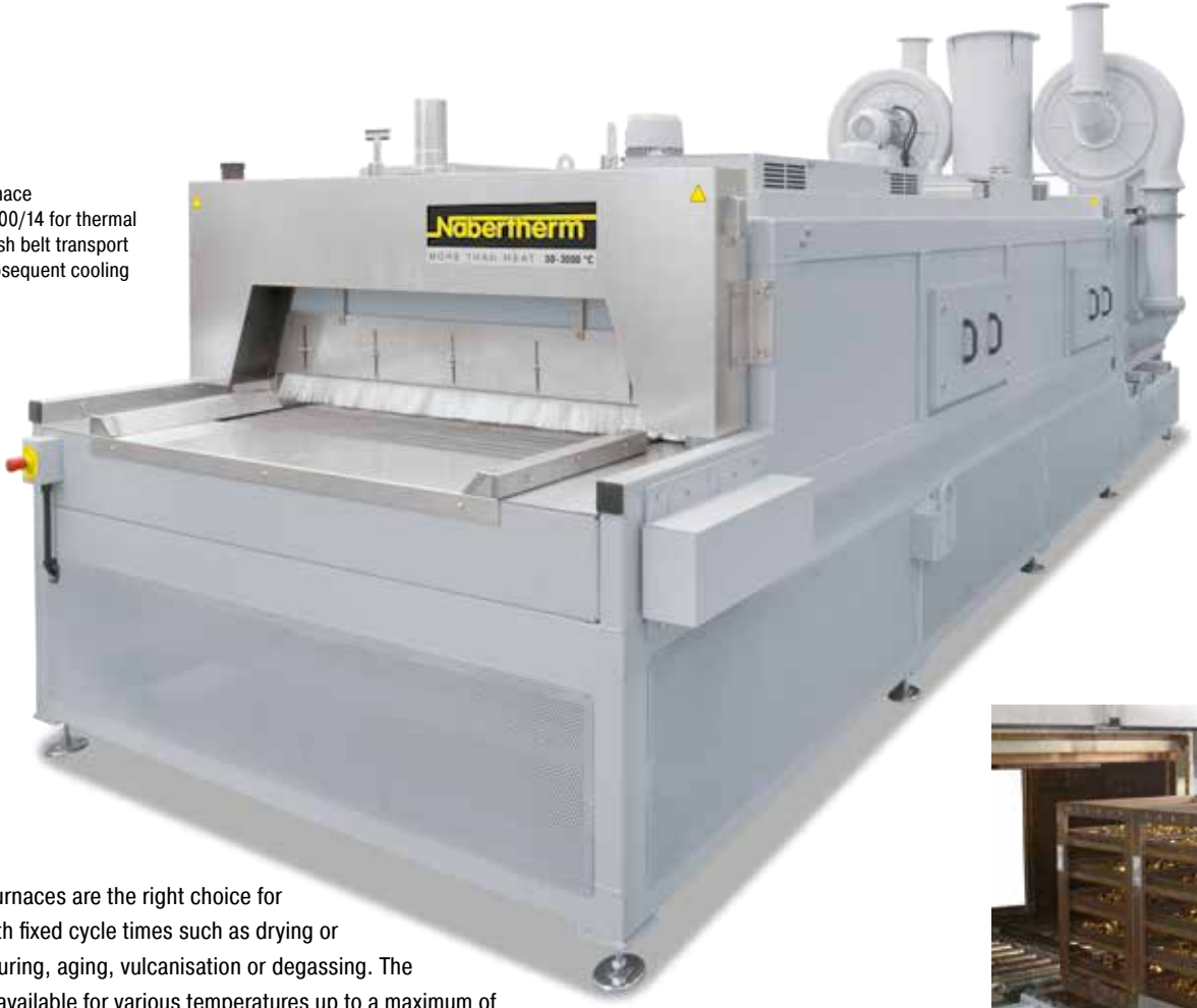
Continuous furnace for bulk materials in baskets
