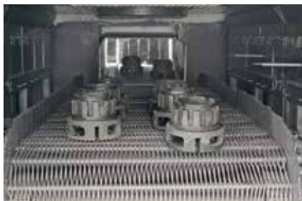
Mesh belt drive in a continuous furnace
