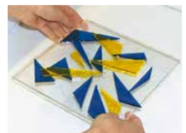
Finished parts out of a fusing furnace
