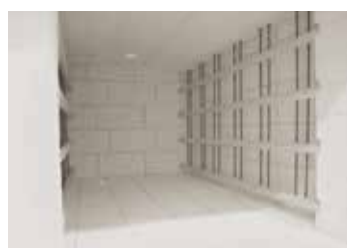
Protection grid in front of heating elements prevent against mechanical damages
