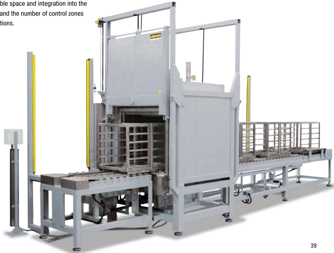
Continuous furnace for bulk materials in baskets
