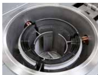
Cylindrical retort with tungsten heating
