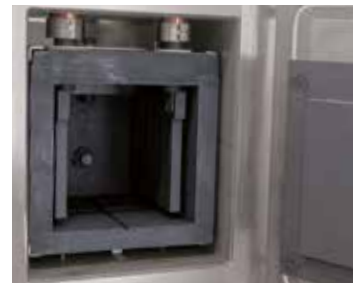
Graphite heating chamber
