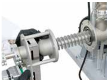
Screw-conveyor with adjustable speed
