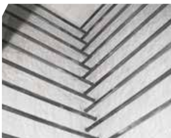
Heating from 4 sides with SiC rods
