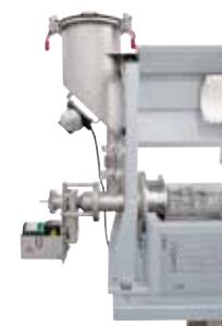
Vibration generator at the charging funnel for improved powder supply
