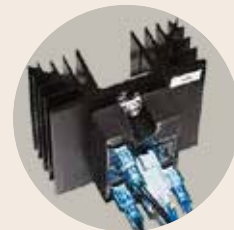
Solid state relays ensure low-noise heater operation
