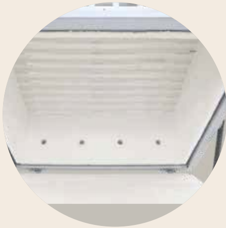
Heating elements in the roof arranged closely next to each other are protected in quartz glass tubes
