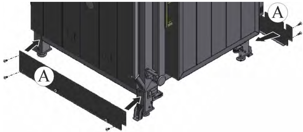
Fig. 37: Assembling the side panels (similar to figure)
