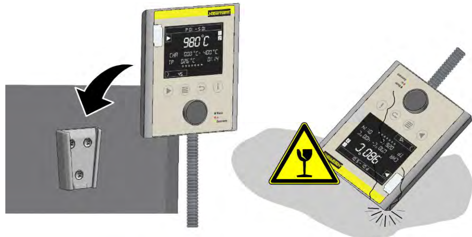
Fig. 42: Place the controller in the holder on the furnace (similar to the picture)
