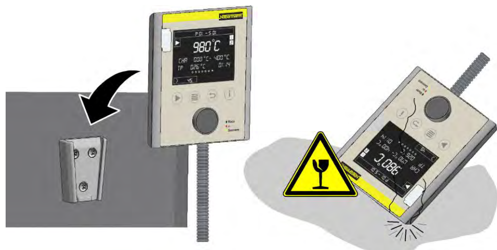
Fig. 62: Place the controller in the holder on the furnace (similar to the picture)
