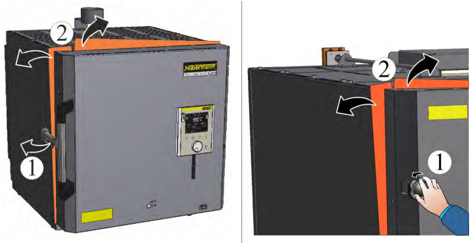
Fig. 12: Example: Removing the transportation protection (similar to picture)
