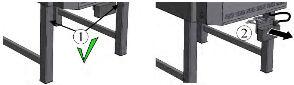
Fig. 39: Remove the bracket from the air inlet flap (similar to picture)
