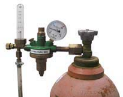
Pressure reducing valve with assembled flow meter
