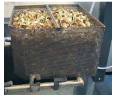
Charging basket for top charging
