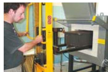
Winch stacker with hardening box and furnace
