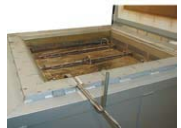
Pit-type furnace S 250/65 with protective gas box for bright annealing
