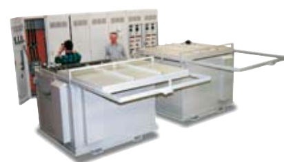
Salt bath plant for annealing of aluminum components in the aircraft industry
