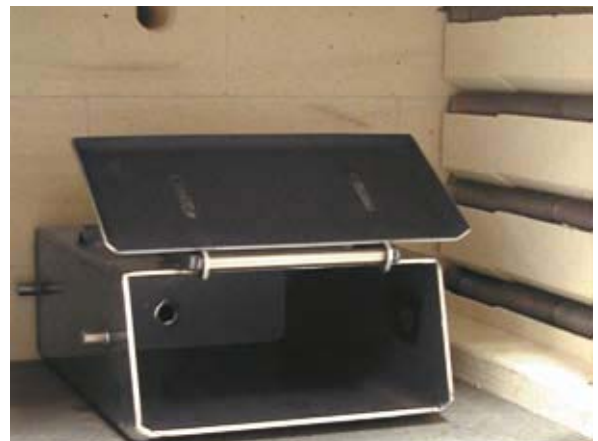
Protective gas box with hinged lid for permanent operation
