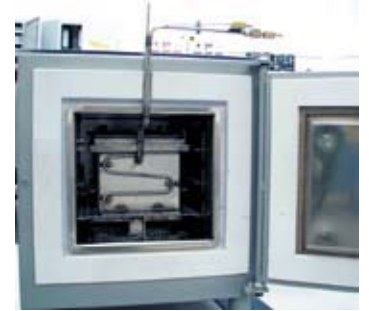
Air circulation furnace with protective gas box
