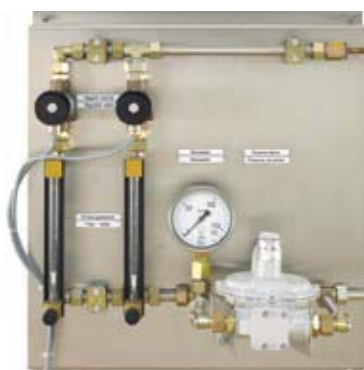
Automatic gas feed system for two flushing quantities
