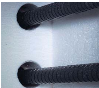
Furnace chamber with high-quality fibre materials and SiC heating rods on both sides of the furnace
