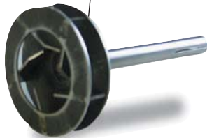
Air-circulation fan in rear wall of furnace
