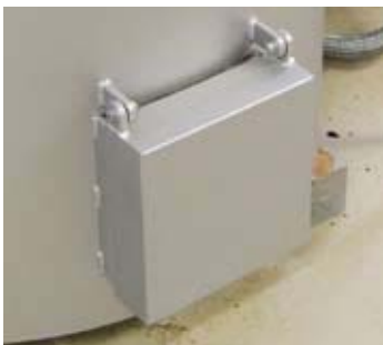
Emergency outlet for the safe draining of melt in case of crucible breakage
