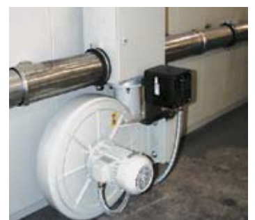
Cooling fan for shorter process times
