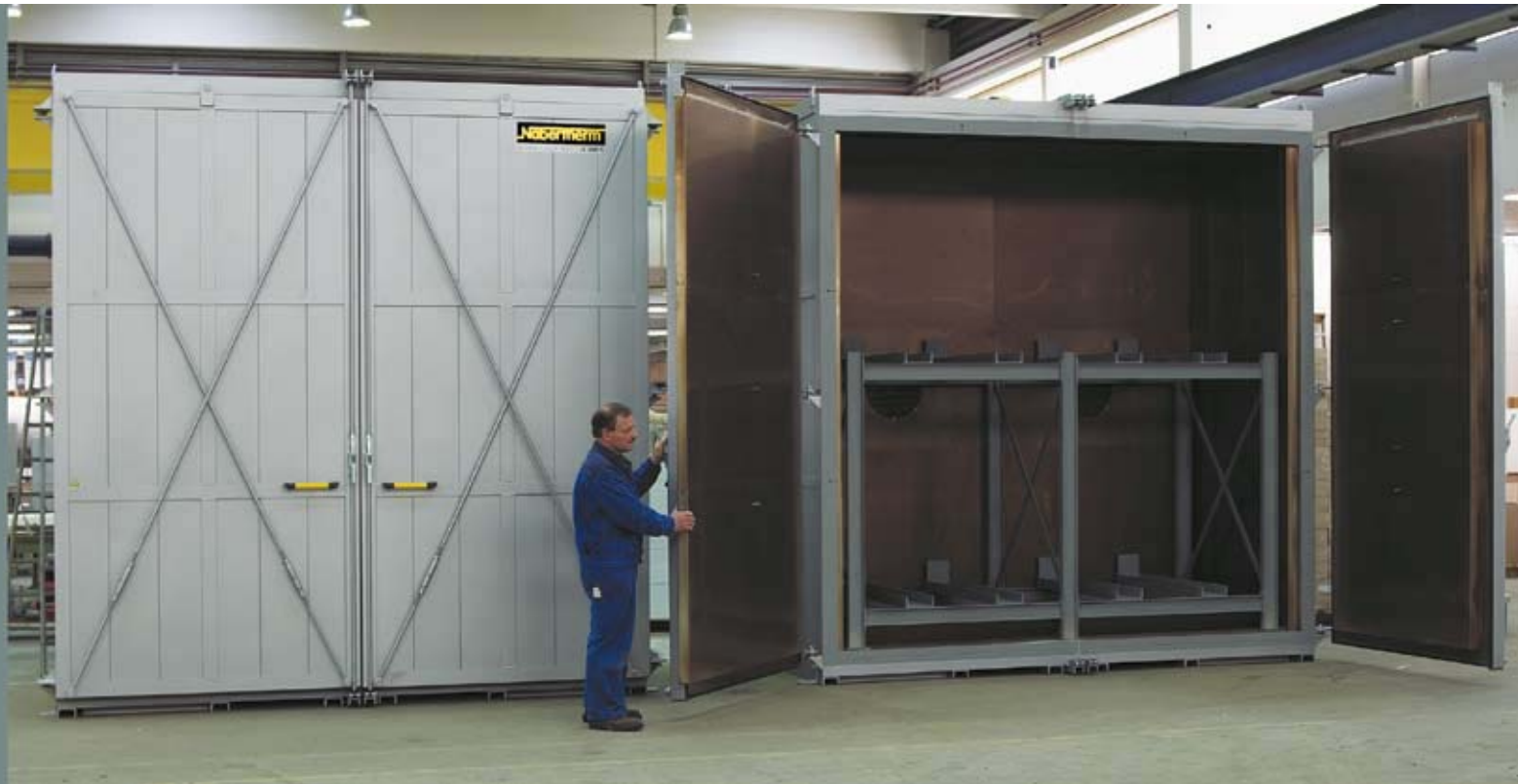
2 x N 12000/26S with charge racks for preheating of molds
