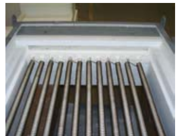
Heating mounted in the lid, simple replacement of the heating elements
