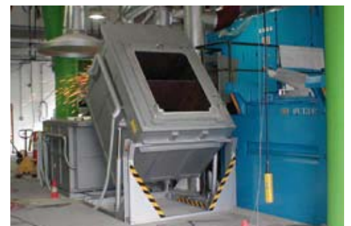
Tilting furnaces for magnesium K 1500/75 S with 1500 liters crucible volume
