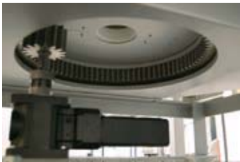
Gear rim drive under the furnace
