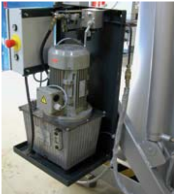
Hydraulics assembly with nonflammable hydraulic fluid
