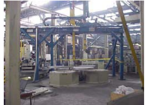
Rotary table system with 3 x T 150/11
