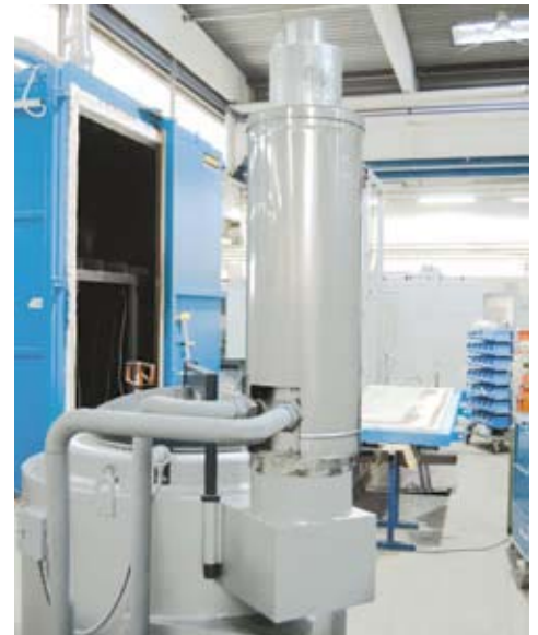
Heat exchanger at gas outlet
