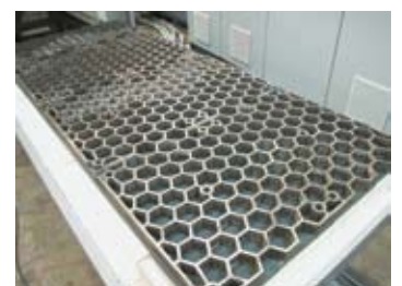
Steel grid on bogie for charging heavy loads
