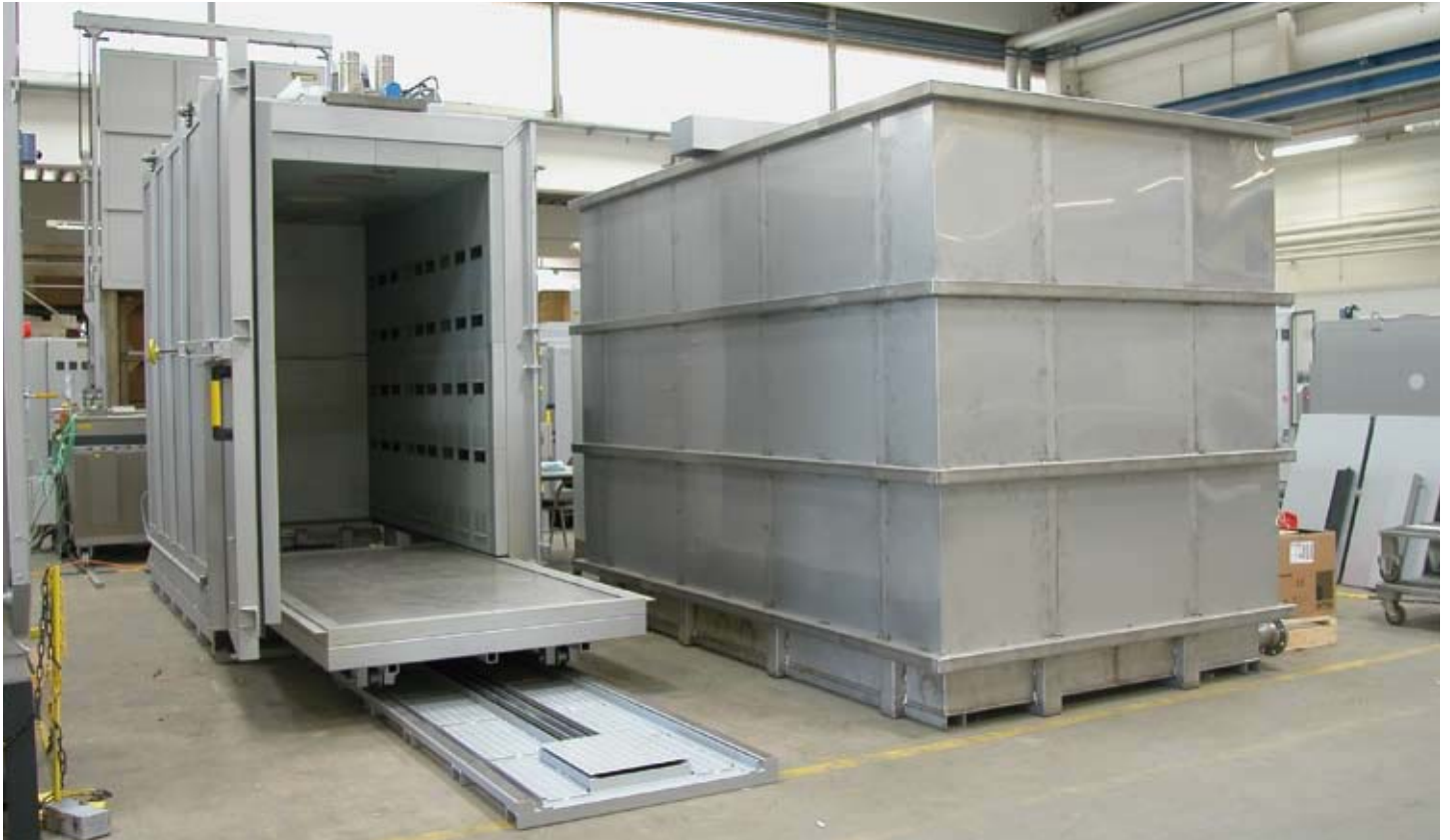
Bogie hearth furnace W 7440/26 AS for solution annealing and water bath WB 24000/S for quenching
