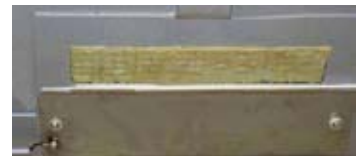
Crucible breakage alarm device under the emergency outlet of a melting furnace
