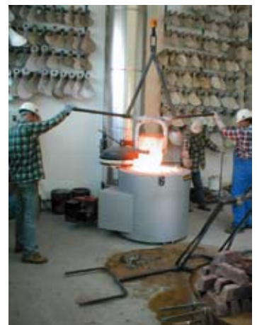
TB 40/14 with crucible pulling feature
