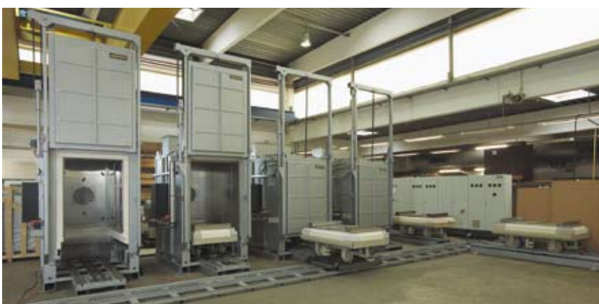
Bogie hearth furnace system with cross-transfer car for automatic bogie exchange
