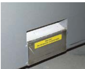
Emergency outlet for the safe draining of melt in case of crucible breakage
