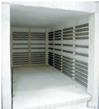
High-quality fibre insulation with corner bricks for shorter heating and cooling times
