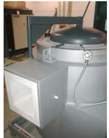
TB 80/12 with side exhaust gas discharge
