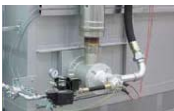
Gas burner firing into a radiant tube for models with gas heating
