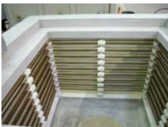
Four side heating for excellent temperature uniformity
