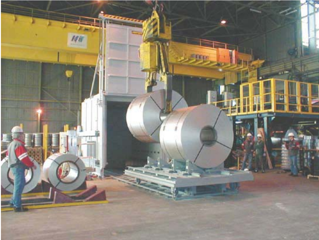
W 21875/26AS bogie hearth furnace for coil preheating, available for charge weights up to 50 tons
