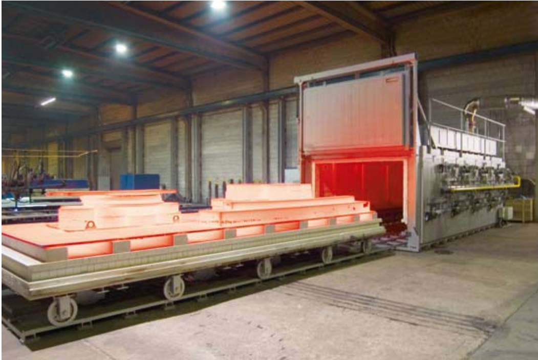
Gas heated bogie hearth furnace WB 14880 S for annealing of large steel parts
