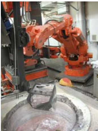
Bale-out of T 650/10 with robot
