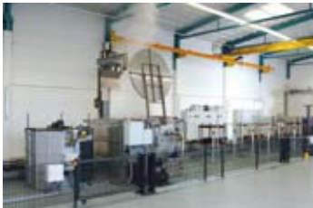
Removal of the charge basket from solution annealing and transfer to water bath
