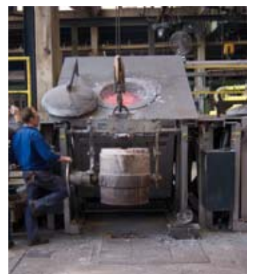
Charging of transport ladle with K 360/12
