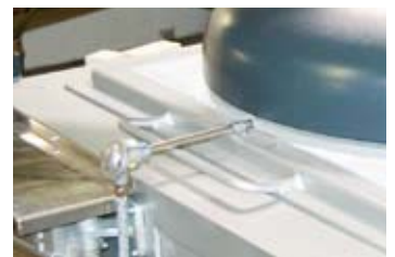
Bath control with thermocouple in the melt.
